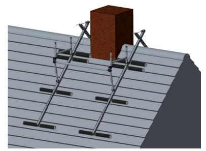
7. Place the extensions at the bottom of the base frames. Make sure that they are adjusted to the maximum length. Secure them at the correct position with a locking pin.
