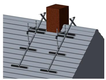
7. Place the extensions on the bottom of the base frames. Make sure that they are adjusted to the maximum length. Secure them at the correct position with a locking pin.
