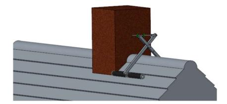
2. First, place the Chimney Access Ridge Stand (CARS Unit) on the ridge of the roof. Depending on the actual dimensions of the roof and the roof tiles used, it should be possible to support the support rollers on the second row of roof tiles. This is to avoid damage to the ridge tiles and the first row of roof tiles at all times. Adjust the Chimney Access Ridge Stand (CARS Unit) with the butterfly nut so that the Chimney Access Ridge Stand (CARS Unit) has the same angle as the roof.
