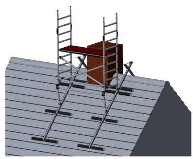
11. Place the platform on the 4th rung of the 8-stage frames. Slide the wind protection locking pins under the load-bearing rungs.
