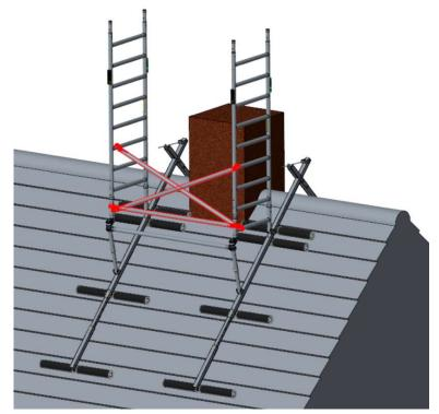
9. Place a horizontal just above the rung of the base frame. Make sure that the openings of the claws point outwards.
