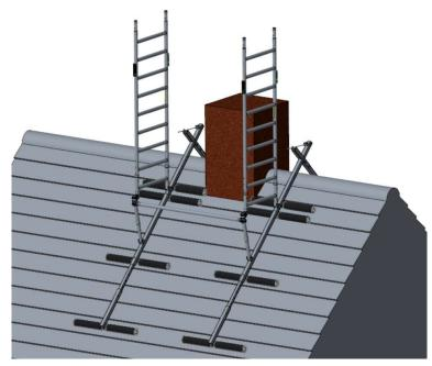
8. Place the 8-stage frames on the coupling pins of the base frames. Secure these with locking pins.
