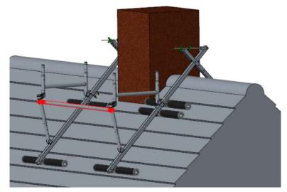
6. Place a horizontal ledger of the same length as the desired platform on the back of the two base frames above the ridges. This will adjust the distance between the two girders to the correct length.
