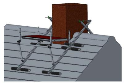
7. Place the platform on the two horizontal rungs of the two base frames. Slide the wind protection locking pins under the load-bearing rungs.
